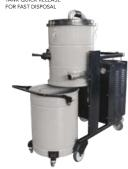
EASIS BT 155 ATEX is the vacuum cleaner that combines power and reliability. Designed and built for constant and continuous use is critical for companies that need a good suction power for vacuuming non-specific dust or debris that can be fine dust.
