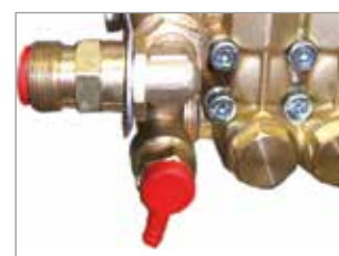
THERMOSTATIC VALVE PROTECTING THE PUMP FROM HIGH TEMPERATURES IN BY-PASS PHASE
